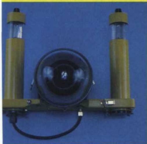
The Light Handle is a custom built electronic flash unit utilizing a unique patented design. The flash reflectors can be rotated to cover three different angles (left-hand flash is detachable).
